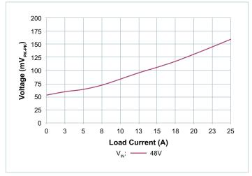
**Figure 11** —  $V_{\text{RIPPLE}}$  vs.  $I_{\text{OUT}}$ : No external  $C_{\text{OUT}}$ , board mounted module, scope setting : 20MHz analog BW
