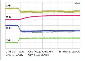
**Figure 14** — OA - 25A transient response:  $C_{IN} = 330\mu F$ ,  $I_{IN}$  measured prior to  $C_{IN}$ , no external  $C_{OUT}$
