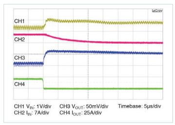
**Figure 15** — 25A – 0A transient response:  $C_{IN} = 330\mu F$ ,  $l_{IN}$  measured prior to  $C_{IN}$  no external  $C_{OUT}$
