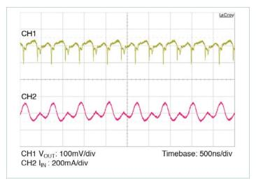
**Figure 12** — Full load ripple, 330μF C<sub>IN</sub>: No external C<sub>OUT</sub>, Board mounted module, scope setting : 20MHz analog BW
